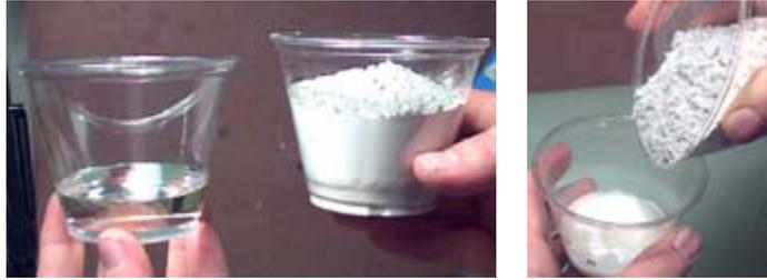
As more plaster sinks to the bottom, it will start to pile up. Keep adding **until you see a lumpy texture form on the surface.**
