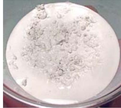
Using a spoon, **gently stir** the plaster to remove the lumps. It should be the **consistency of a thin milk shake** or pancake batter. Getting the consistency just right will take a few casts.
