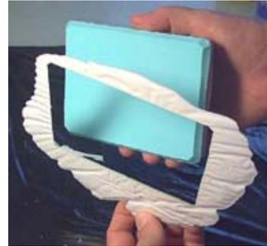
**Remove the glass from the mold.** If you sprayed enough mold release on the glass, it should pop off easily.
