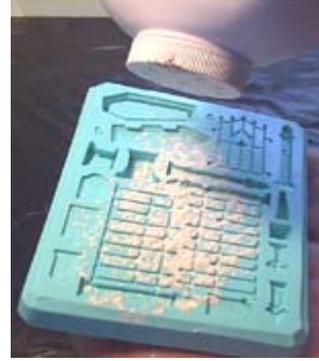
5. **Hold the mold over a trash can.** Tilt the mold and **tap the sides** to spread the talc around. Turn the mold a  $\frac{1}{4}$  turn and tap the next side. Continue all the way around until the talc covers all of the pieces in the mold.
