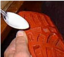
When pouring plaster into the small pieces with deep recesses, flex the mold to stretch out the area. This will leave fewer narrow crevices to form air bubbles.
