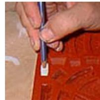
Also, after you pour the plaster in, use a toothpick or dull pencil and trace around the shape to release air bubbles. Mixing the plaster **slightly** thinner will also help. Be sure to tap the mold often to release air bubbles.
