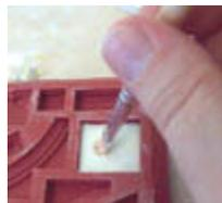
When pouring into the small decorative floor tiles use an old stiff bristled paint brush and push it around to force the air bubbles out. It's very difficult to remove the air bubbles otherwise.
