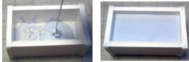
6. Tear the box off of the mold and remove the original sculpture. Usually, the sculpture gets destroyed while taking it out of the mold.
