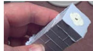
5. Now for the hard part. I didn't consider how difficult it would be to remove the original from the mold. After a bit of forcing, it came out. A straight or fluted pillar would have come out easier. Regardless, I got it out and the mold works fine.
