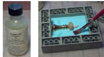
10. Pour rubber over the other half. When cured, remove the legos and peel them apart. The two halves should fit together perfectly and the keyways will help them line up.
