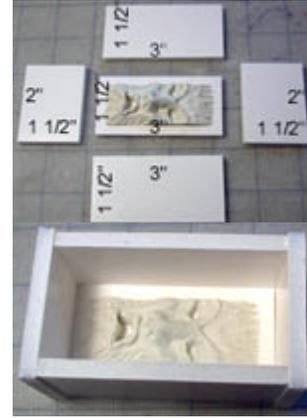
2. The kind of silicone I'm using for this mold is purchased from Micromark ([www.micromark.com](http://www.micromark.com)). It's called ONE-TO-ONE/RAPID mold making rubber. To use this material you measure out equal parts of A and B, which means you don't need a scale to weigh the parts.
