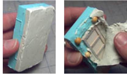
7. Coat the rubber completely with a layer of mold release compound. This will keep the two halves of the mold from sticking together. Try to avoid painting the door.
