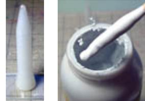
2. Thin the material down with water until it's the consistency of heavy cream. Paint the material over your object and remove any air bubbles that form on the surface by blowing on it.
