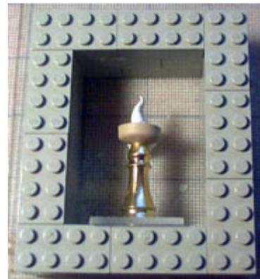
To make a 2-piece mold, you have to submerge the bottom half of the object in something, so the rubber will only cover one half at a time.
