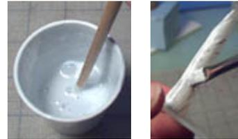
3. Let the first coat **dry completely** (about 4 hrs). The second coat is full strength. You should put at least 4 coats (letting it dry completely between coats) for a complete mold.
