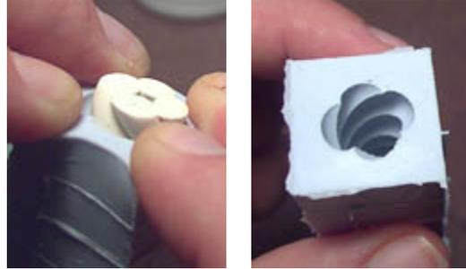
6. Mount the skull base on a piece of plexiglass or wood. This time I'm going to make a box out of wood. It really doesn't matter what you make the box out of, as long as it will contain the rubber.
