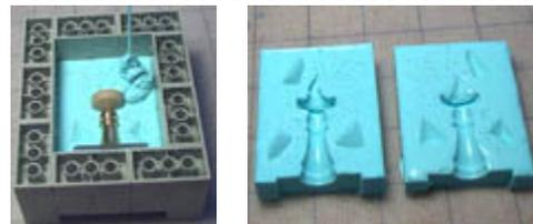
11. Before putting the halves together, **coat them with talcum powder**. This will help remove air bubbles. Place a piece of heavy stock on both sides of the mold (I'm using foam core board). Put a couple of rubber bands around it. **Don't get them too tight** or they'll distort the mold while casting.
