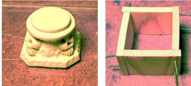
7. As before, paint with a coat of rubber. Place the wooden box over top and seal the outside edges with modeling clay. Pour the rubber mixture over top.
