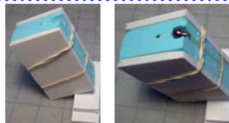
The door came out OK except for a large air bubble that formed at the neck where the material was poured in.
