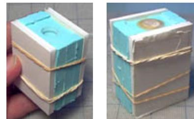
12. Open the mold to reveal the finished cast. It will probably need some trimming.
