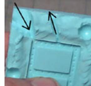
10. **Coat the insides of the mold with talcum powder.** Place a piece of heavy stock on both sides of the mold. Put a couple of rubber bands around it. Don't get them too tight.
